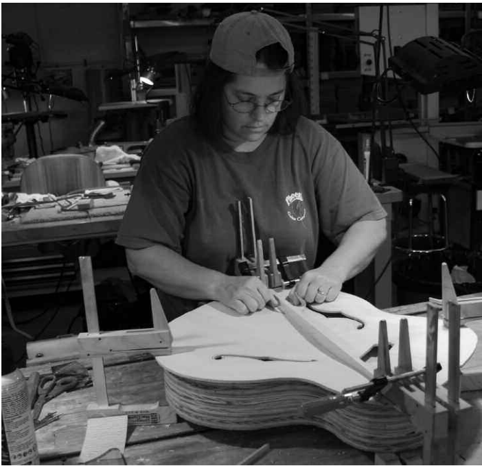
Diana sands the underside of a brace as she fits the brace to the contour of the top prior to gluing the braces down.
