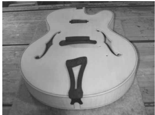
This is the guitar body basically done. Binding has been glued on and bridge and tailpiece are shown.
