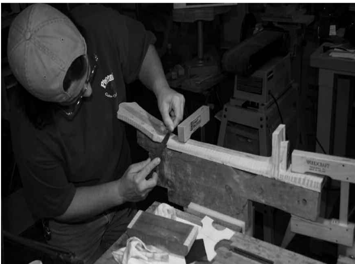
Diana working on the final neck profile with a file.
