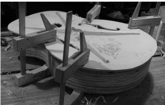
The underside of the top, braces mostly carved, still some sanding to do.
